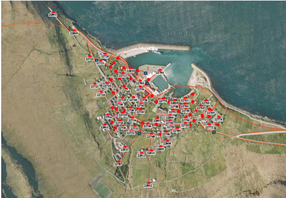
Figure 4.2 Electric grids in and through Leirvík. The orange line is 20 kV (from www.kortal.fo )
