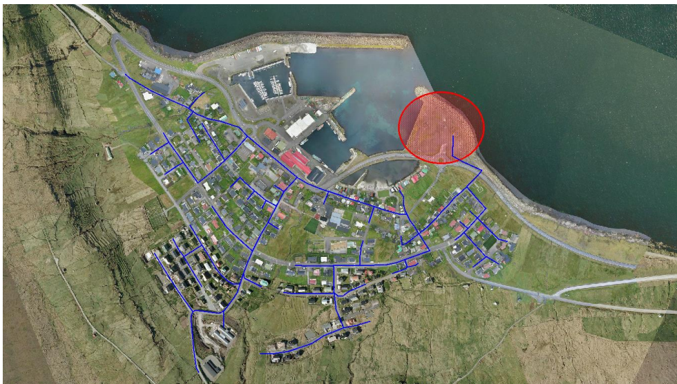
Figure 8.1 Overview of the brine network and the placement of the seawater intake.
