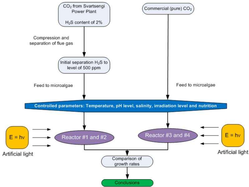
Figure 27. Schematic flow chart of geothermal biomitigation experiment by utilizing blue green microalgae.
