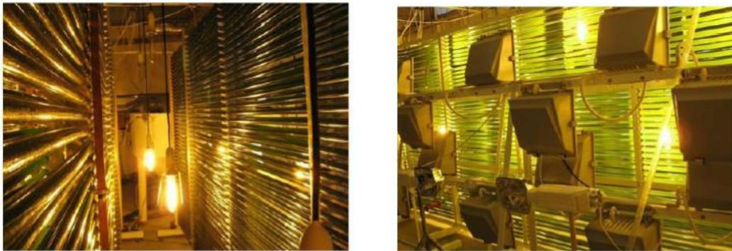
Fig. 3. Pilot scale reactor of total volume 1000 Ltrs.
