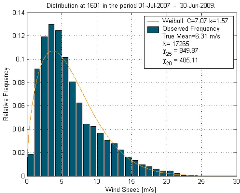
Figure 4 Distribution of wind speed and calculated weibull distribution for 6101 Nanortalik. The distribution is calculated using the Risø anemometer at 48.8 m and NRG #200P wind wane at 41.4 m height.
