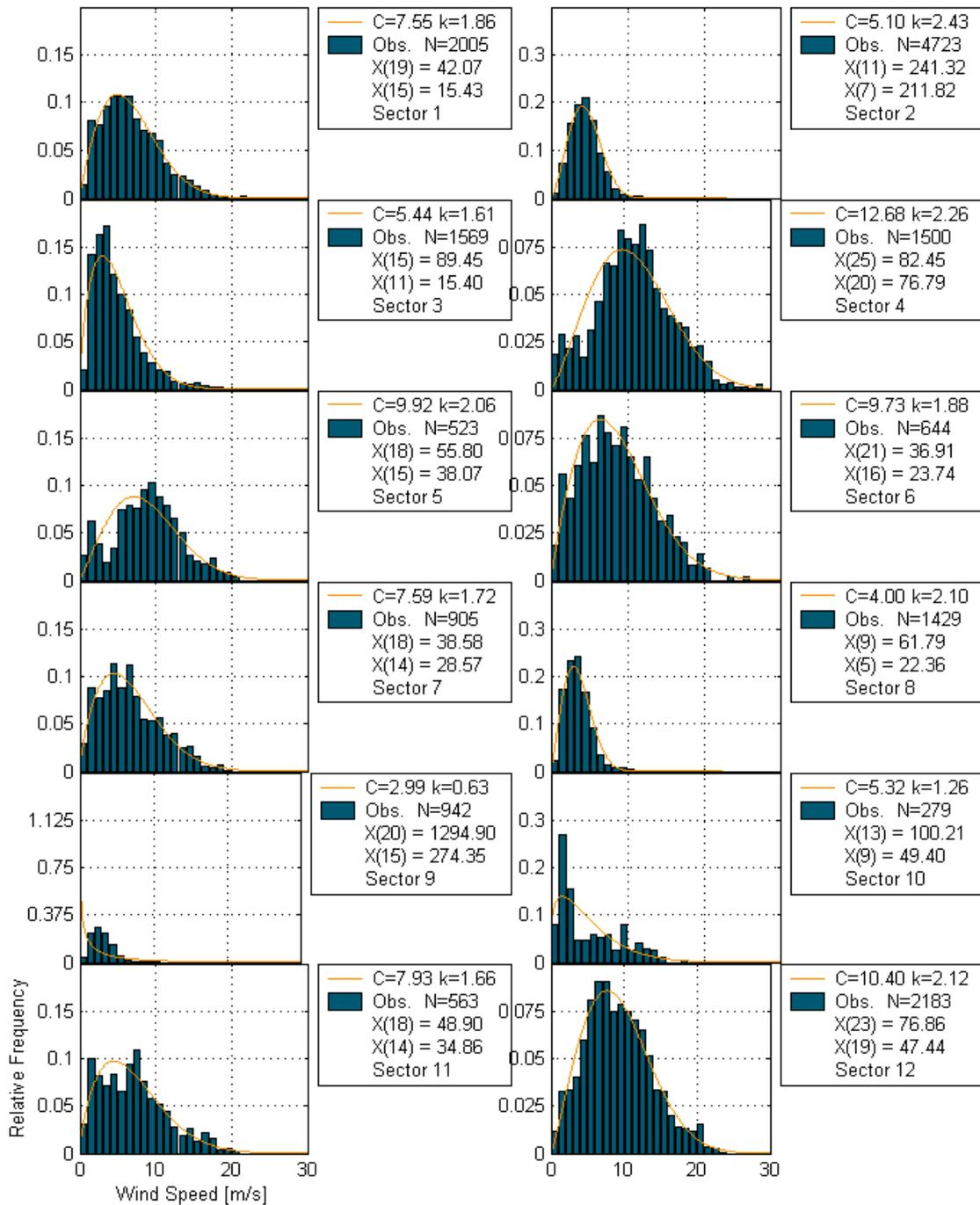
Figure 3 Distribution of wind speed for 12 sectors, and estimated weibull distribution for each sector. Sector 1 is north ( $345^{\circ}$ - $15^{\circ}$ ), each sector covers  $30^{\circ}$  in clockwise direction. The distribution is calculated using the Risø anemometer at 48.8 m and NRG #200P wind wane at 41.4 m height.
