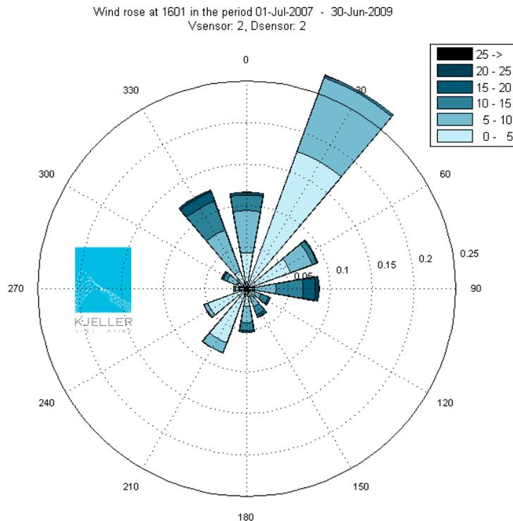
**Figure 2** Wind rose for 6101 Nanortalik based on data for July 1 2007 - August 2 2009. The wind rose is plotted using the Risø anemometer at 48.8 m and NRG #200P wind wane at 41.4 m height.
