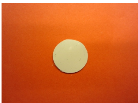
Figure 9: Image of a green BCZY tape of diameter 16 mm.
