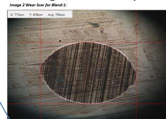
\*wear scar diameter (WSD) (ASTM D7566-12a standard (2013))
