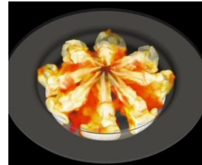
LES of methanol spray flame in Scania D13 PPC engine
