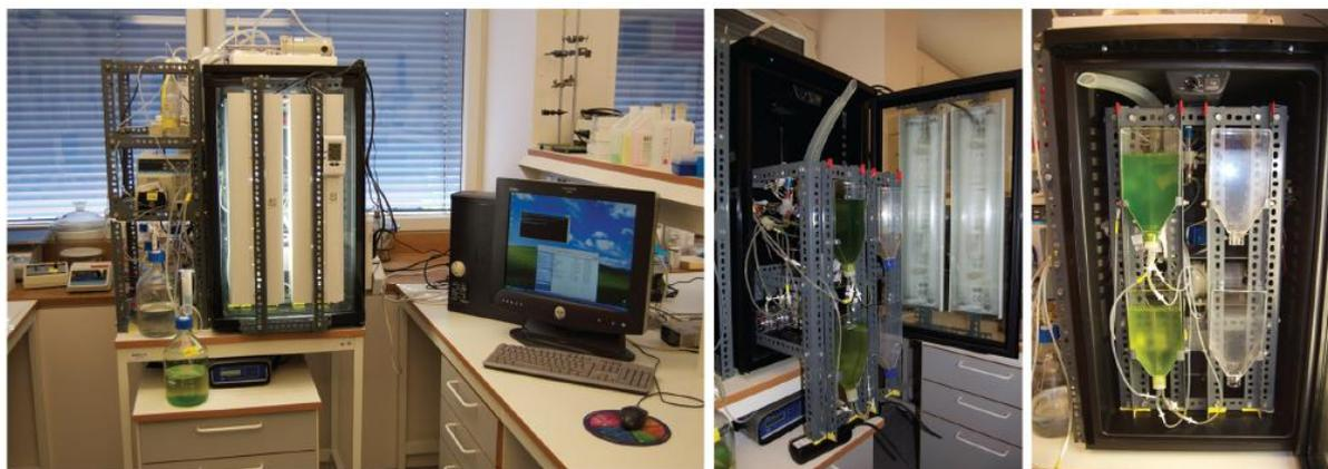
Figure IV.2. Incubator with  $\text{CO}_2$  delivery system and data logging computer (left), internal rack with gas traps and pH electrodes (middle), chemostats with  $\text{CO}_2$ -repleted stage at top and  $\text{CO}_2$ -depleted stage at bottom (right).
