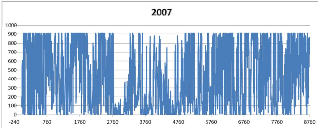
Figure 9 Wind power production per 0.9 MW Enercon turbine for the year 2007. X-axes: hours per year, y-axes: power production in kW
