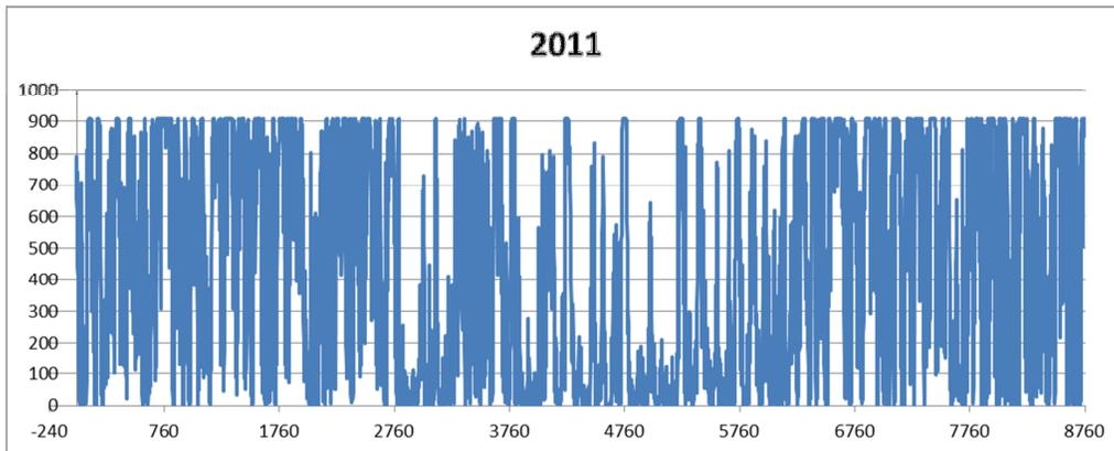
Figure 10 Wind power production per 0.9 MW Enercon turbine for the year 2011. X-axes: hours per year, y-axes: power production in kW
