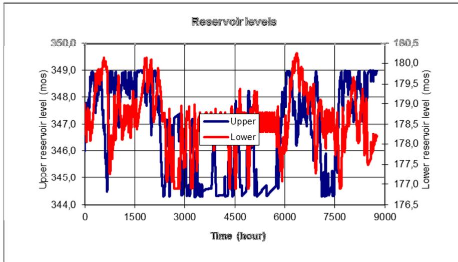
Figure 12 Reservoir levels for the "base case", with 2,5 m<sup>3</sup>/s turbine capacity in the PSPP, with an unchanged reservoir volume (upper reservoir: 550 000 m<sup>3</sup>, lower reservoir: 725 000 m<sup>3</sup>). The read curve show the water level in the lower reservoir, the blue curve shows the water level in the upper reservoir for the year 2012.
