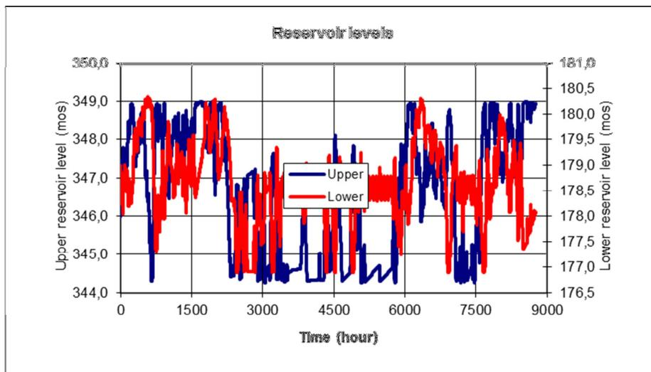
Figure 13 Reservoir levels with 3,125 m<sup>3</sup>/s turbine capacity in the PSPP, with an unchanged reservoir volume (upper reservoir: 550 000 m<sup>3</sup>, lower reservoir: 725 000 m<sup>3</sup>). The read curve show the water level in the lower reservoir, the blue curve shows the water level in the upper reservoir for the year 2012. As the larger turbine empties the upper reservoir more quickly, the reservoir size is more completely filled.
