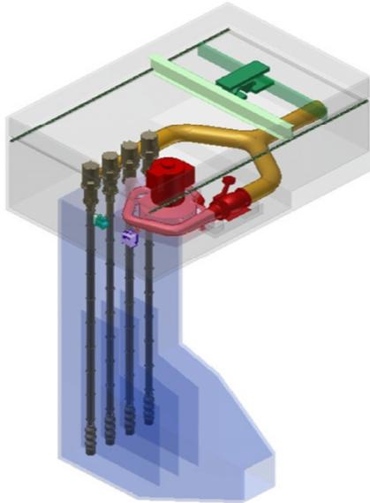
*Figure 2 Power house overview. 3D-sketch of suggested concept with one Pelton turbine and 4 pumps*
