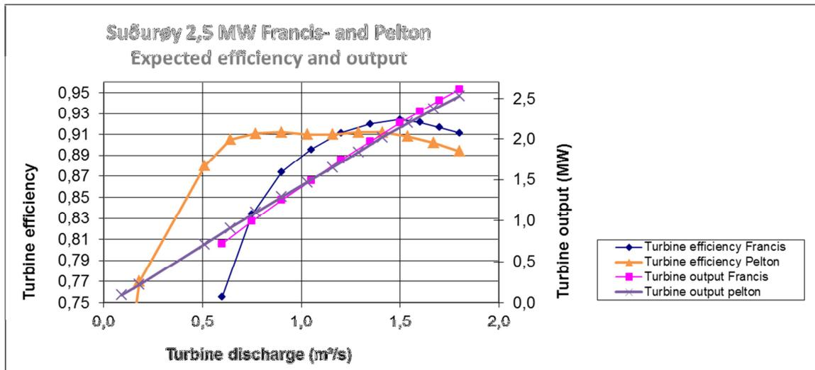
Figure 5 Typical turbine efficiency and -output diagram.
