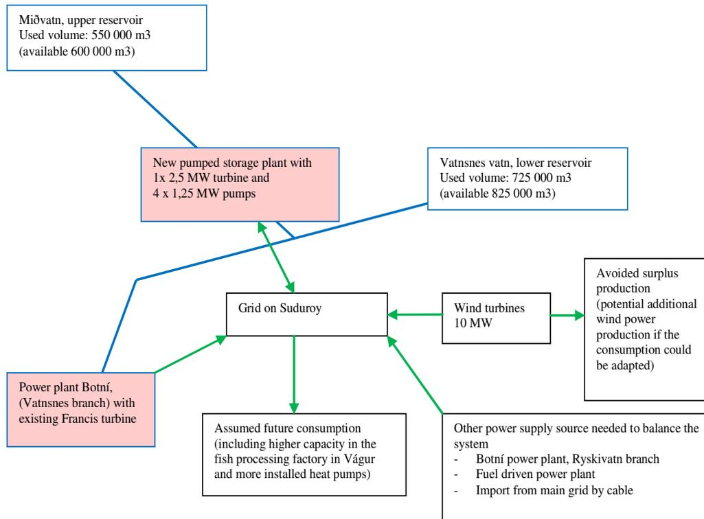
Figure 6 Elements of the model that was used for simulating power production and demand on Suðuroy (base case). The blue lines indicate the parts of the pumped storage plant and the Vatnsnes-branch of the power plant in Botní. The green lines symbolize the exchange of power.
