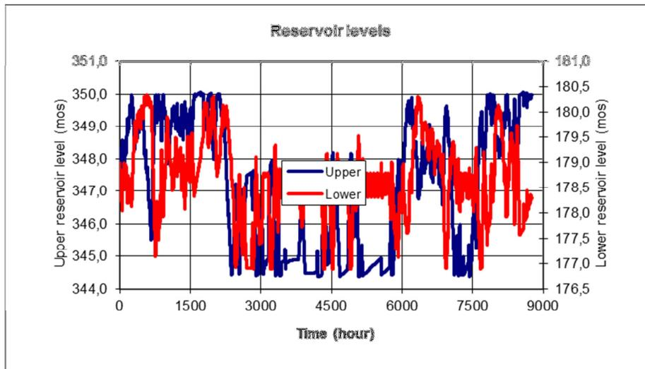
Figure 14 Reservoir levels with 3,125 m<sup>3</sup>/s turbine capacity in the PSPP and with a higher upper reservoir volume (725 000 m<sup>3</sup>), resulting the same reservoir capacity in the lower and the upper reservoir. The read curve show the water level in the lower reservoir, the blue curve shows the water level in the upper reservoir for the year 2012. In times with much inflow, the reservoir reaches it maximum water level also with the slightly larger reservoir.
