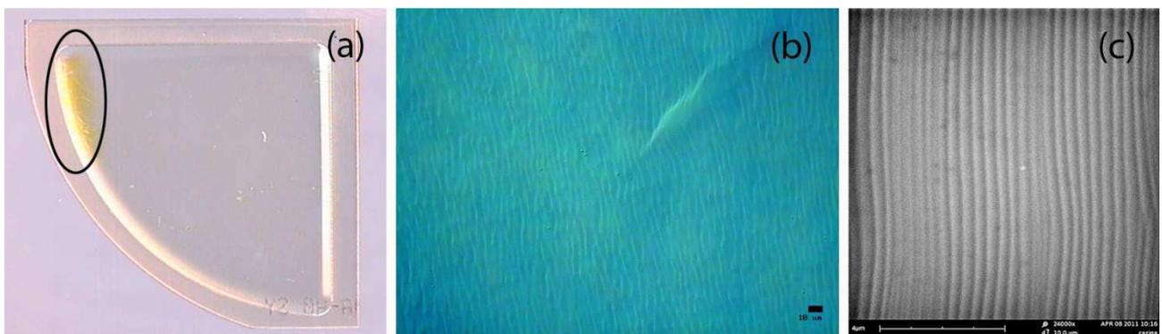
*Fig. 10 Surfaces of samples grown on quarter of 2 inch wafer with 50 ppm B doping: (a) overall figure, a 3C area is marked by a ring; (b) optical microscopy image, scale 10  $\mu\text{m}$ ; (c) SEM image, scale 4  $\mu\text{m}$ .*
