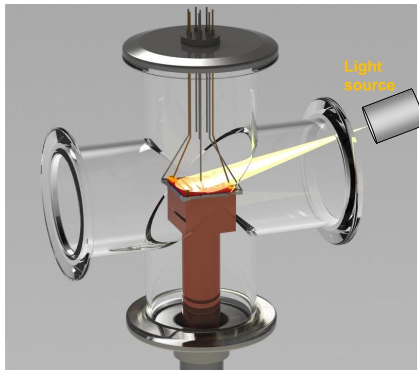
**Through port with optical feedthrough**
