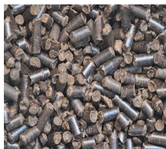
'Black wood pellets' used in the test campaign November 2017. Delivered by Arbaflame AS.
