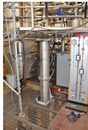
New sub-system for cooling and flue-gas clean-up at the Chalmers CLC test unit.
