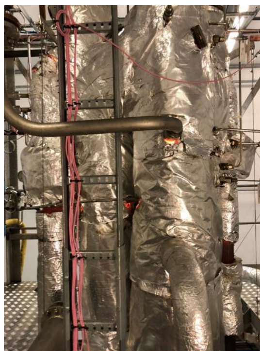
Upper part of reactors at operating temperature (1000 oC) during SINTEF ER CLC testing Q3 2018
