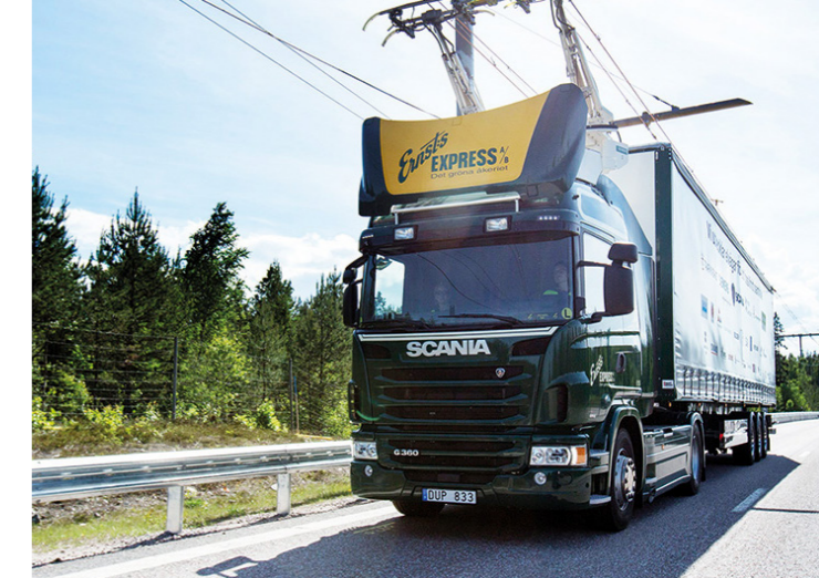
Electric road with overhead lines. Scania's and Siemens' project outside Gävle, Sweden. (Picture: Scania)
