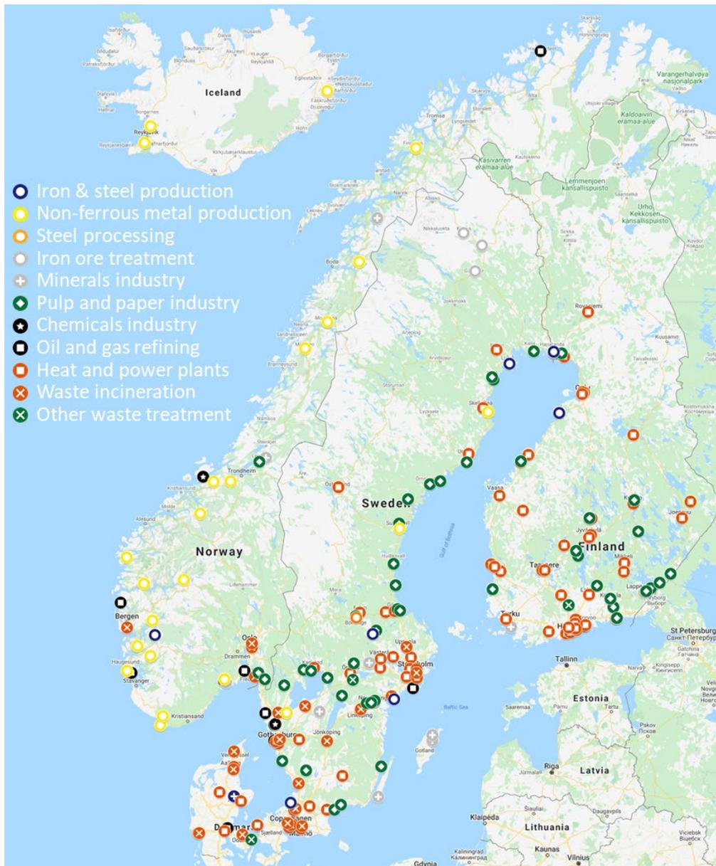
Figure 4.2. The 232 investigated sites for e-fuel production, categorised by industrial activity according to the E-PRTR classification.
