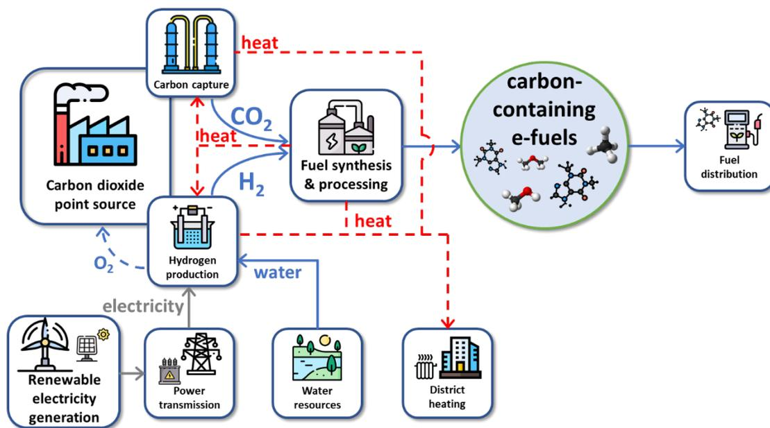
Figure 4.1. Illustration of production of carbon-containing e-fuels at large-scale CO<sub>2</sub> point sources.
