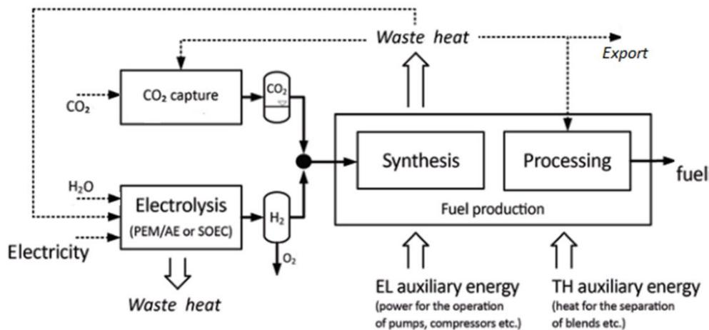
Figure 1.1 Principle flow chart for the e-fuel or P2X process, converting electricity and hydrogen into various types of fuels (based on [1])
