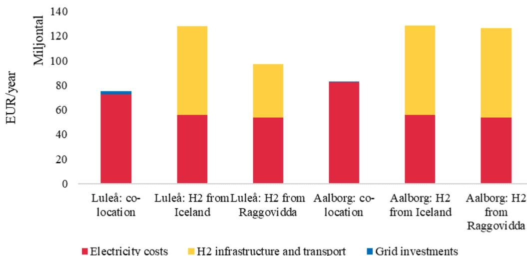
Figure 4.5: Cost of hydrogen production.
