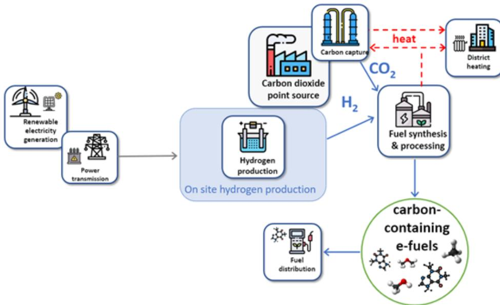
Figure 4.3: Onsite hydrogen production
