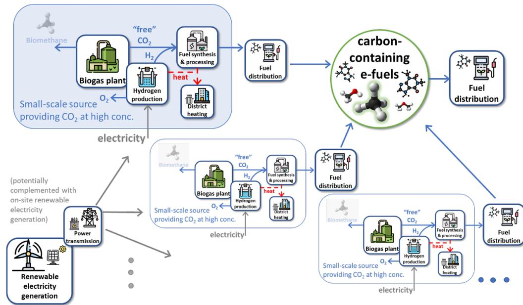
Figure 4.6: Illustration of e-fuel production scenario at multiple small-scale sites.
